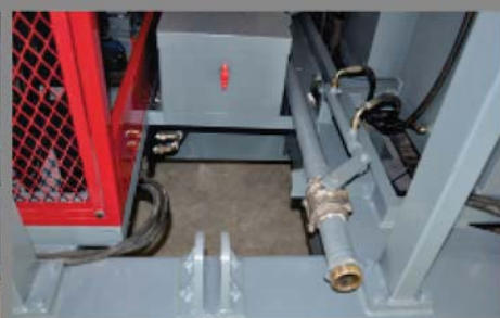
Open/close of drilling fluid supply is controlled by hydraulic cylinder.
