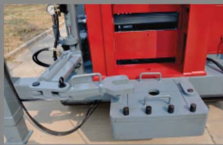
Clamping system can be adjusted for height
