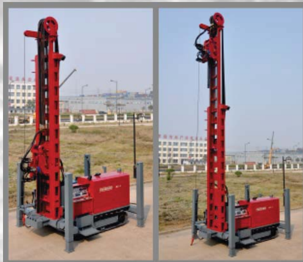
Telescoping mast, possible to use 6.1 m length drill rod
