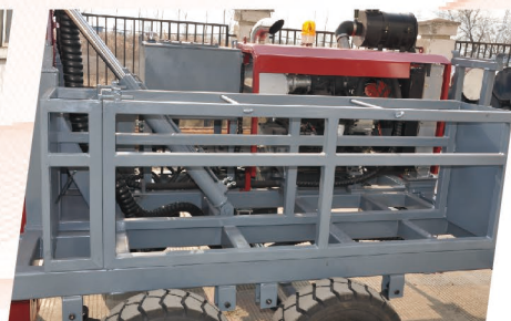
Utilises a Rod Box system for a tidier operation
