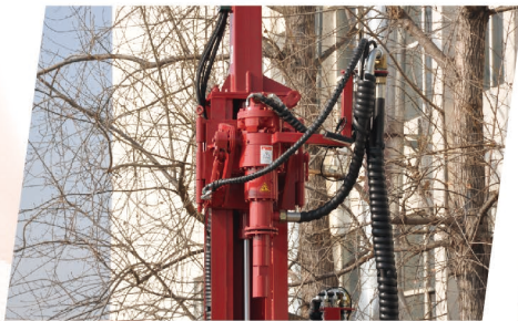
Powerful power head, top-drive rod system and big diameter core water swivel
