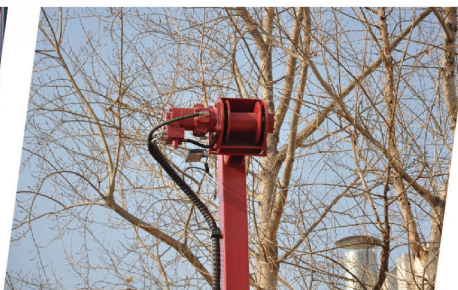
Large capacity hoist of 62Kn
