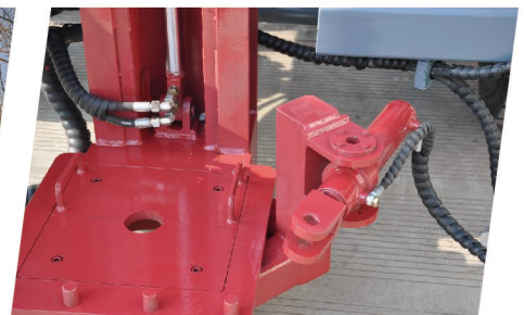
Height adjustable clamping system
