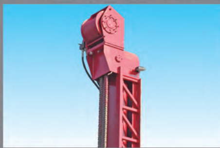
The crane set up on the top of the mast. The capacity of hoist is 2 ton.
