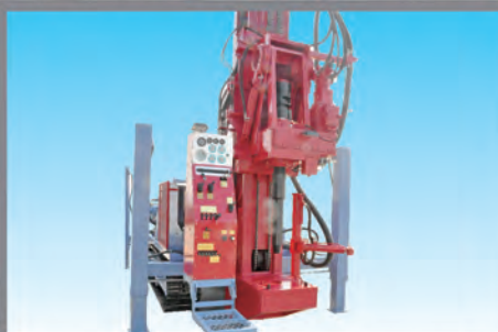
Clamping system can be adjusted for height
