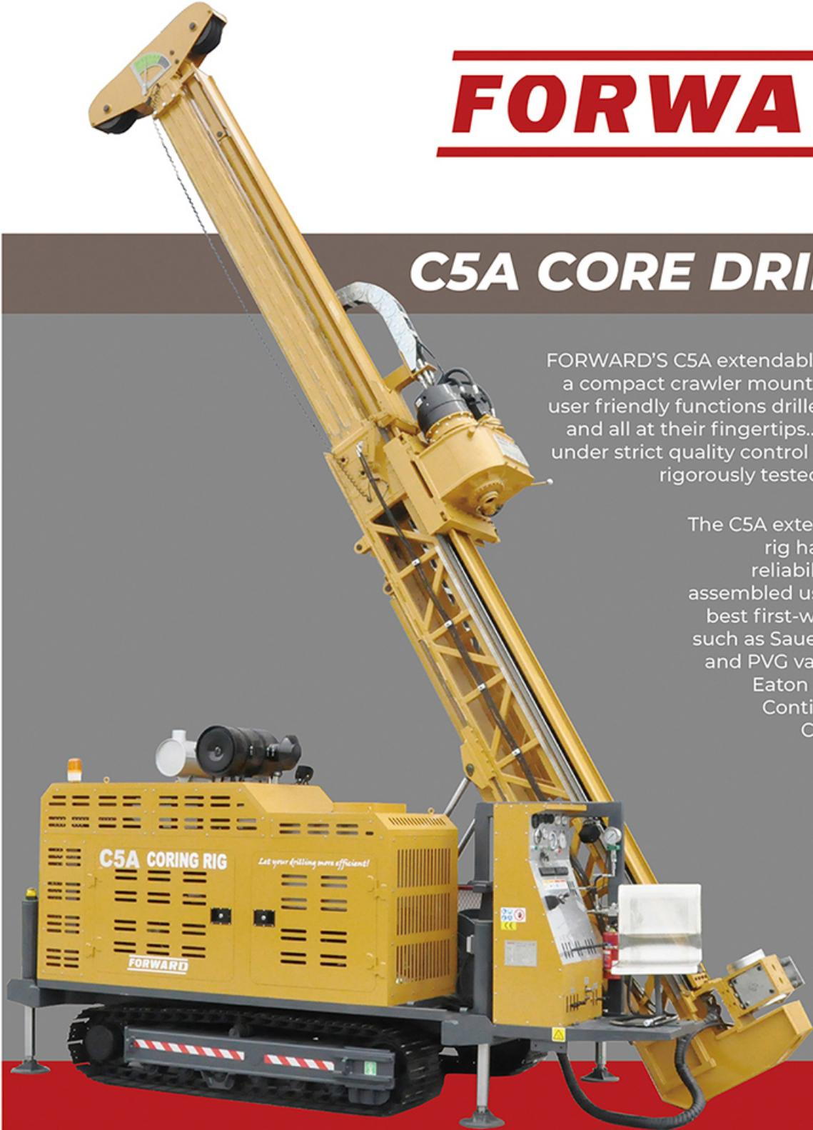
The C5A is extremely compact but has depth capabilities that are only found on much larger rigs. AND, it drives straight into a shipping container which makes it extremely economical to ship anywhere in the world.
