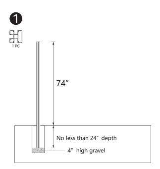
1. Dig a hole for post, 12" diameter 28" depth; Fill 4" gravel into the hole; Put the post on the gravel.
