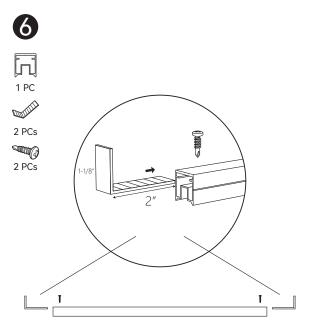
6. Insert L shape bracket into top rail channel;
