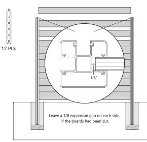
5. Stack 12 WPC fence boards between the posts.
