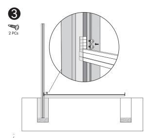
3. Insert the bottom rail into one post's channel; Insert the bottom rail into the other post's channel; Mark the location of the other post; Dig a hole for the other post, 12" diameter 28" depth;
