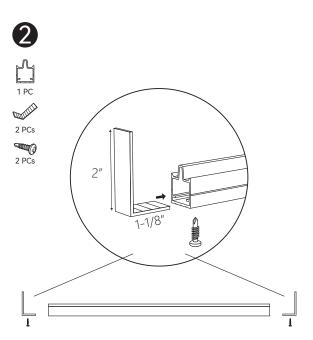
2. Insert the "L" shape bracket into the bottom rail channel; Make sure insert the shorer side (1-1/8") into the channel; Secure the self tapping screw;
