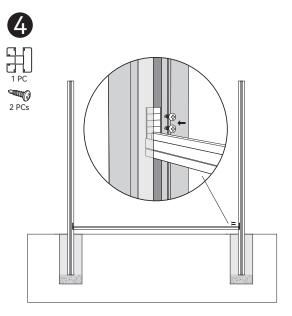
4. Pour the cement into the hole; Double level the post; Set aside untill cement dry.
